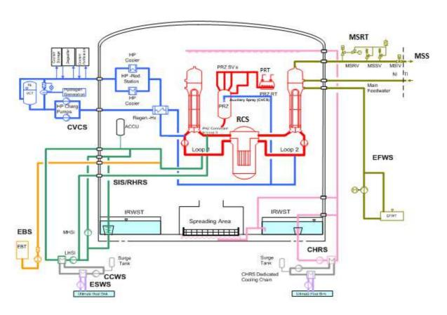
CCWS: Component Cooling Water System
