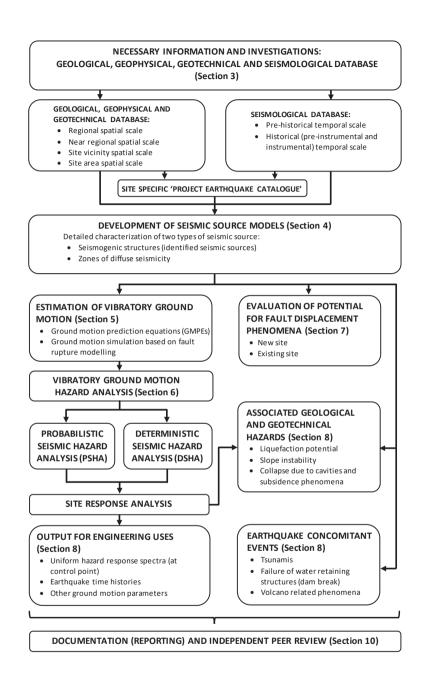
FIG. 1. Flow chart showing the seismic hazard assessment process for nuclear installations.
