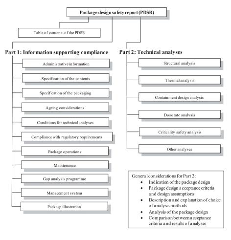
FIG. 1. Structure and contents of a package design safety report.
