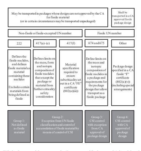
FIG. 2. Overview of the provisions for the transport of fissile material (adapted from Ref. [9], where CA — competent authority; CSI — criticality safety index; FE — fissile-excepted; F — fissile). Paragraph numbers are from the Transport Regulations [1].
