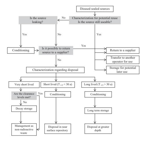
FIG. 3. Flow diagram illustrating the main steps in the management of disused sealed sources.
