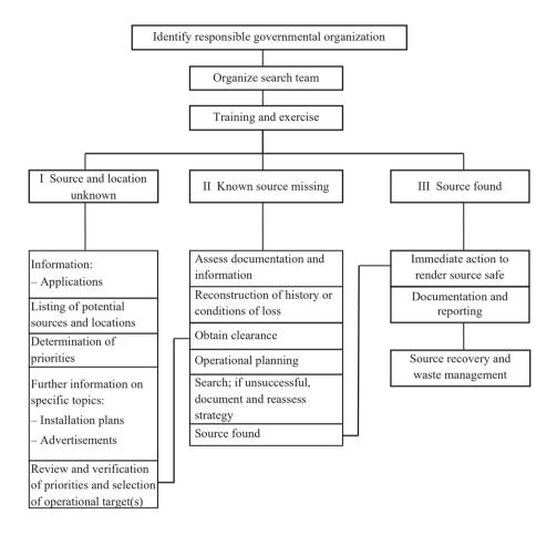
FIG. II–1. An example of a strategy for the identification and location of disused sealed radioactive sources.
