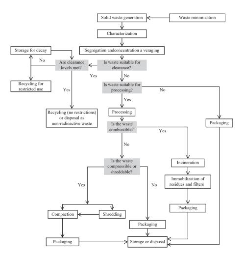
FIG. 1. Flow diagram illustrating the main steps in the management of solid radioactive waste.
