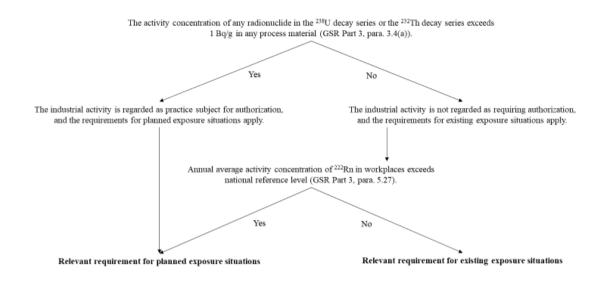
FIG. 1. Flow chart illustrating how to select approach for protection of workers against radon exposure based either on the activity concentration in material of uranium or thorium decay series or activity concentration of radon.
