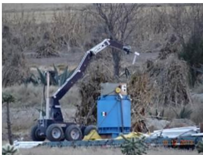
Fig. I-16. Placing the source in the container using the robot (Credit: CNSNS).
