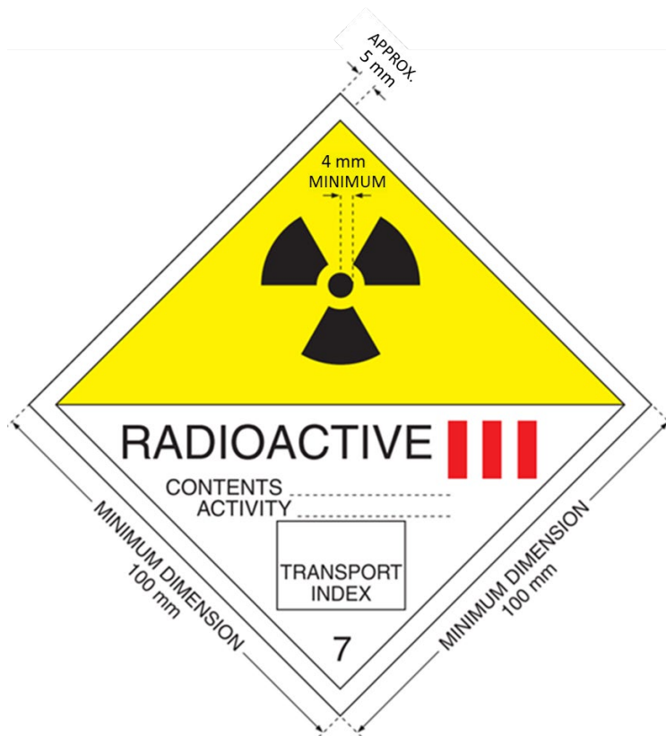
FIG. 4. Category III-YELLOW label. The background colour of the upper half of the label shall be yellow and the lower half white, the colour of the trefoil and the printing shall be black, and the colour of the category bars shall be red.
