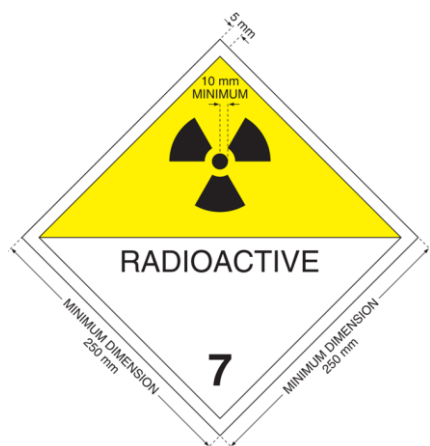
FIG. 6. Placard. Except as permitted by para. 571, minimum dimensions shall be as shown; when different dimensions are used, the relative proportions shall be maintained. The number '7' shall not be less than 25 mm high. The background colour of the upper half of the placard shall be yellow and of the lower half white, the colour of the trefoil and the printing shall be black. The use of the word "RADIOACTIVE" in the bottom half is optional, to allow the alternative use of this placard to display the appropriate UN number for the consignment radioactive material .
