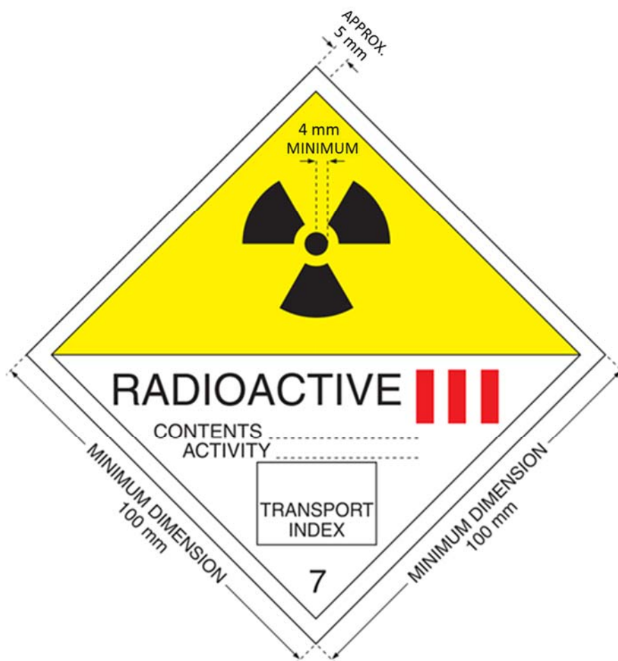
FIG. 4. Category III-YELLOW label. The background colour of the upper half of the label shall be yellow and the lower half white, the colour of the trefoil and the printing shall be black, and the colour of the category bars shall be red.
