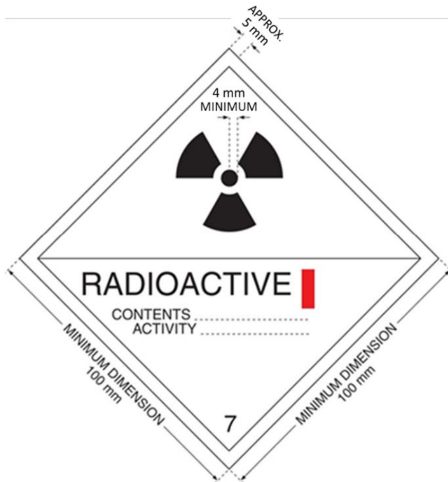
FIG. 2. Category I-WHITE label. The background colour of the label shall be white, the colour of the trefoil and the printing shall be black, and the colour of the category bar shall be red.
