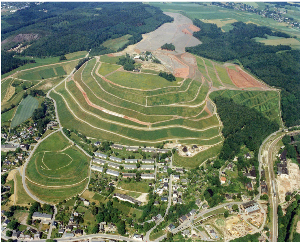
FIG. I-4 Waste rock pile and shaft n° 382 in 2005, showing that final cover is nearly finished ( Archive Wismut GmbH ).
