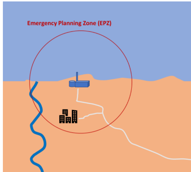
FIG. 2. Example of a site with a physical barrier (river) without an alternative evacuation route in another direction – site potentially unsuitable if a bridge is not constructed or an alternative evacuation route is not available.
