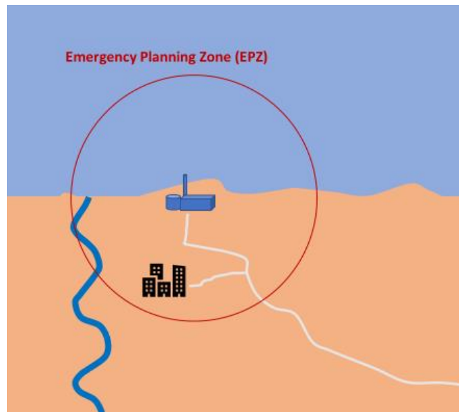
FIG. 2. Example of a site with a physical barrier (river) without an alternative evacuation route in another direction. The site potentially is unsuitable if unless a bridge is not constructed or an alternative evacuation route is not made available.
