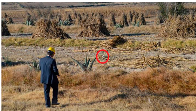
FIG. I-15. Exposed radioactive source (courtesy of Federal Commission for Electricity of Mexico).
