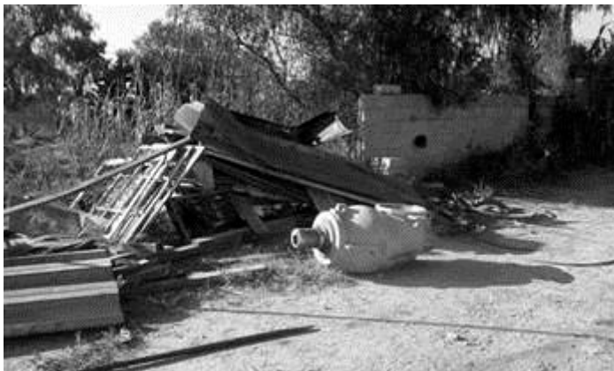
FIG. I-14. The empty shielding of the radioactive source (courtesy of the CNSNS).
