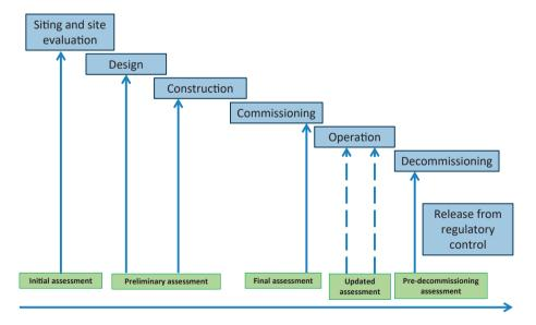
FIG. 1. Stages in the lifetime of a nuclear installation when a prospective radiological environmental impact assessment might provide input into the authorization process (adapted from SSG-12 [33]).
