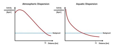
*FIG. I–1. Typical patterns of environmental activity concentrations as a result of atmospheric and aquatic dispersion of discharges from facilities and activities in normal operation.*
