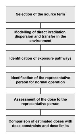
FIG. 2. Components of a radiological environmental impact assessment for protection of the public in normal operation. (This figure is not intended as a detailed step by step procedure and is presented to illustrate the elements of the assessment and facilitate its description.)
