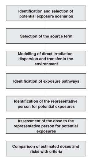
FIG. 3. Components of an assessment for consideration of potential exposures. (The figure is not intended as a detailed step by step procedure and is presented to illustrate the elements of the assessment and facilitate its description.)
