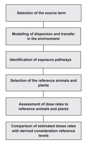
FIG. I–2. Components of a generic assessment for protection of flora and fauna in normal operation. (The figure is not intended as a detailed step by step procedure and is presented to illustrate the elements of the assessment and facilitate its description.)
