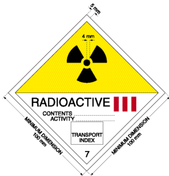
FIG. 4. Category III-YELLOW label. The minimum width of the line inside the edge forming the diamond shall be 2 mm. The background colour of the upper half of the label shall be yellow and the lower half white, the colour of the trefoil and the printing shall be black, and the colour of the category bars shall be red.
