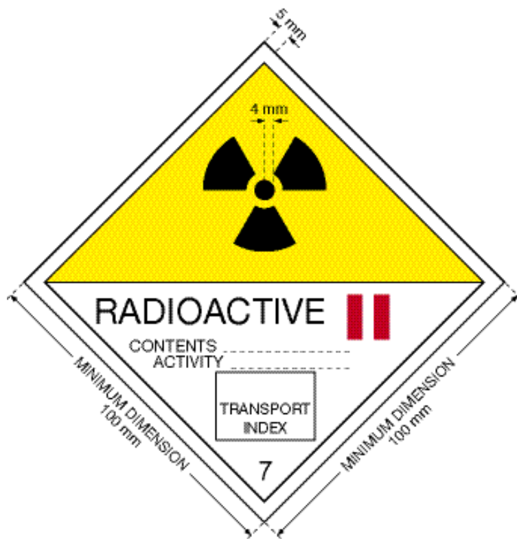
FIG. 3. Category II-YELLOW label. The minimum width of the line inside the edge forming the diamond shall be 2 mm. The background colour of the upper half of the label shall be yellow and the lower half white, the colour of the trefoil and the printing shall be black, and the colour of the category bars shall be red.
