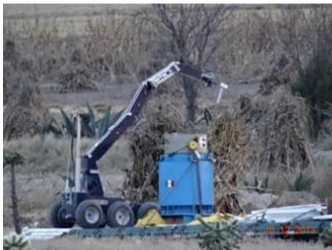
Fig. I-16. Placing the source in the container using the robot (Credit: CNSNS).
