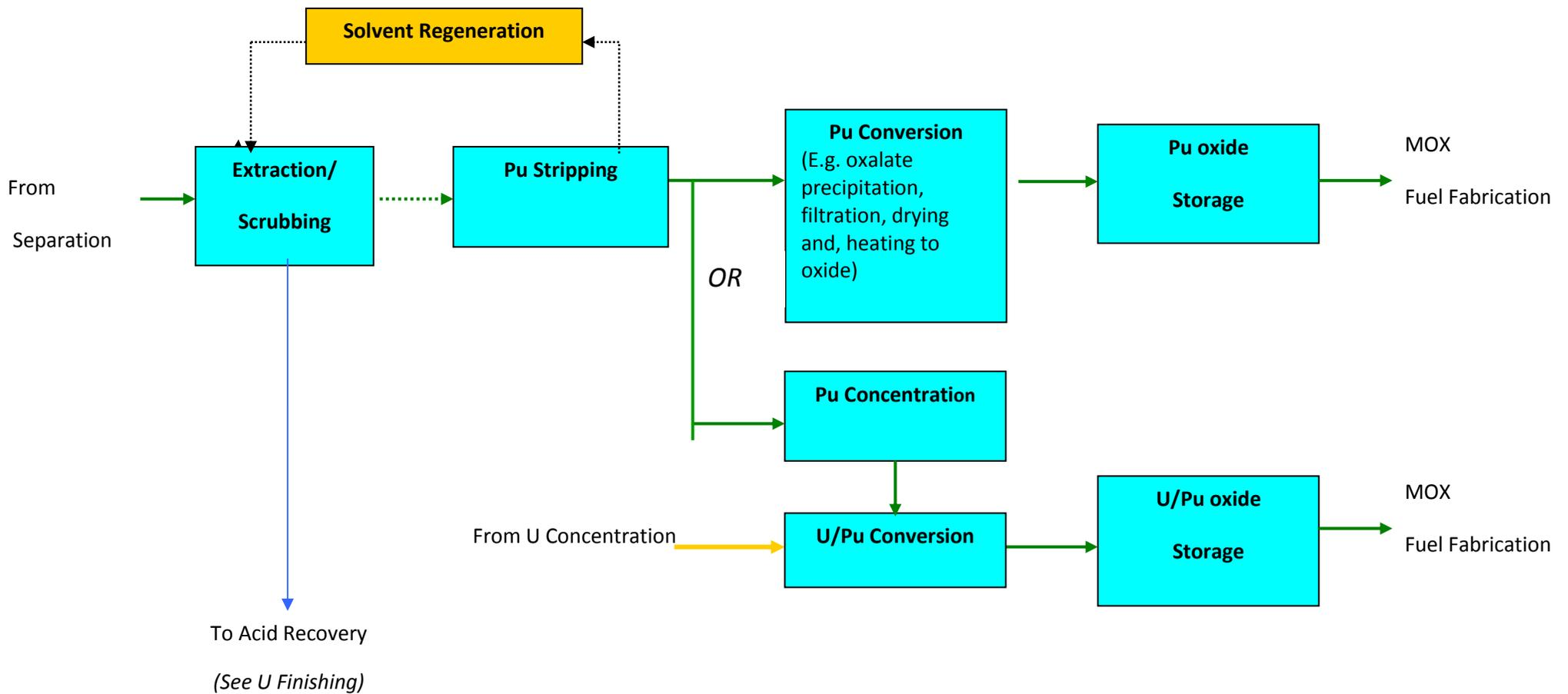
Fig. I-4. Plutonium finishing at a reprocessing facility.
