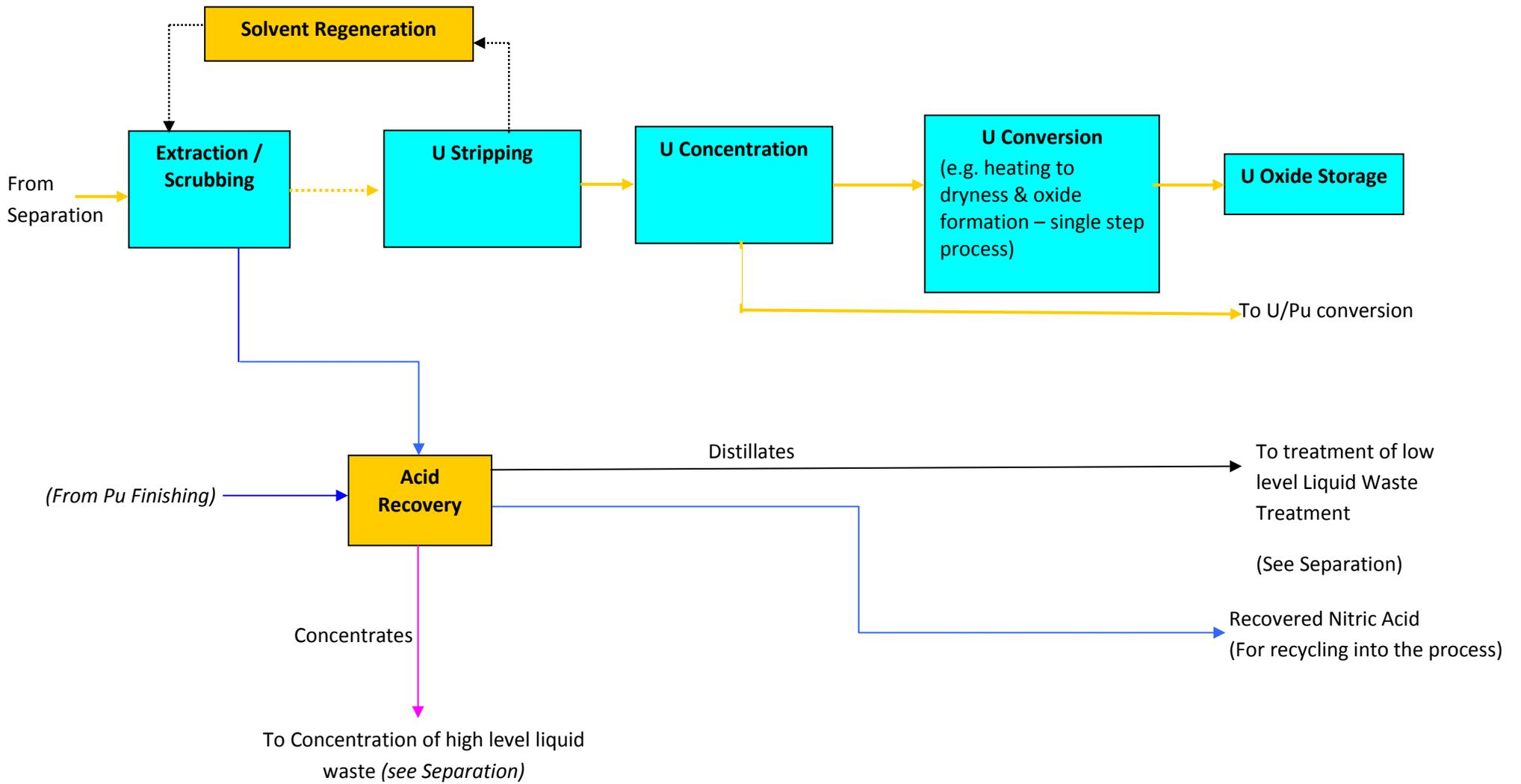
Fig. I-3. Uranium finishing at a reprocessing facility.
