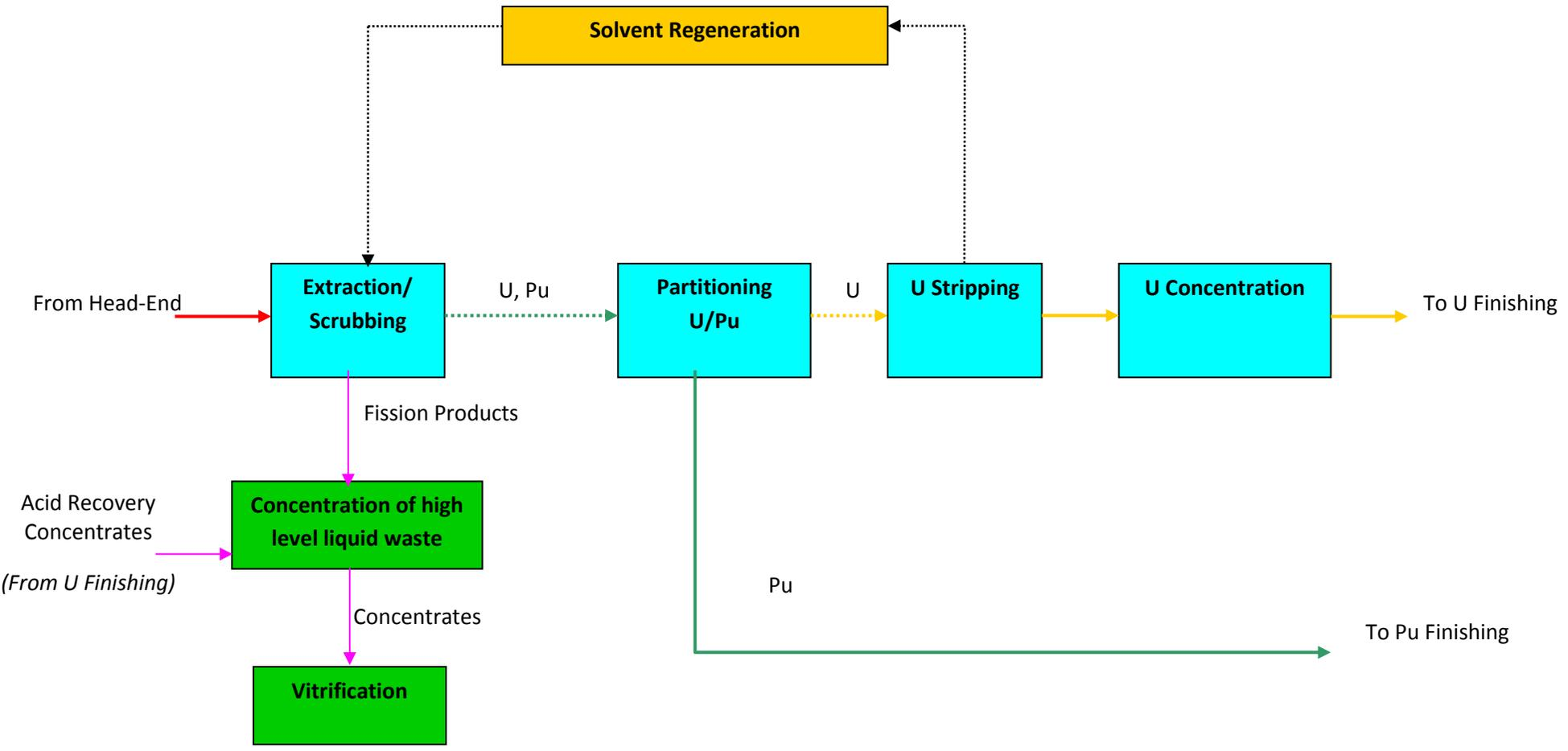
Fig. I-2. Separation of uranium and plutonium at a reprocessing facility.
