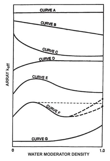
FIG. VI.1. Typical plots of array  $k_{\rm eff}$  versus interspersed water moderator density.
