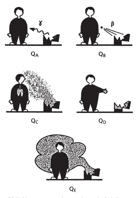
FIG. 1.1. Schematic representation of exposure pathways employed in the  ${\it Q}$  system.
