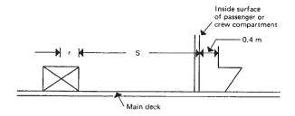
FIG. III.3. Typical configuration of main deck stowage on a combi or cargo aircraft.
