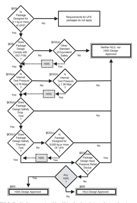
FIG. 2. Graphical representation of the additional package design and approval requirements for uranium hexafluoride.
