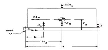
FIG. IV.3. Force diagram used in analysis.
