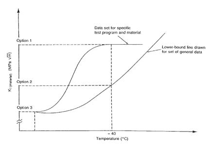
FIG. V.2. Relative values of  $K_{I(mat)}$  measurements based on the selection of options 1, 2 or 3.
