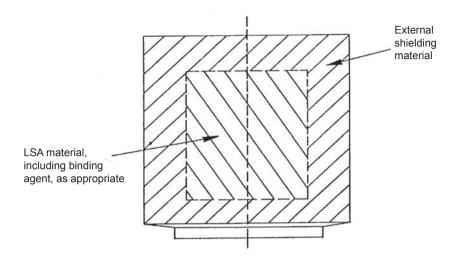
FIG. 1. LSA material surrounded by a cylindrical volume of non-radioactive shielding material
