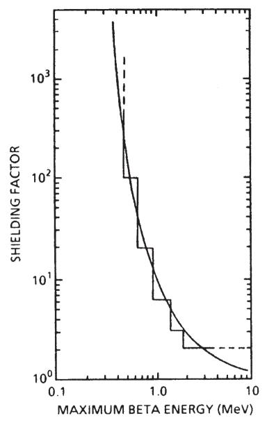
FIG. 1.2. Shielding factor as a function of beta energy. Shielding factor =  $e^{\mu d}$ ,  $\mu = 0.017 \times E_{\beta_{max}}^{1.14}$ ,  $d = 150 \text{ mg/cm}^2$ .
