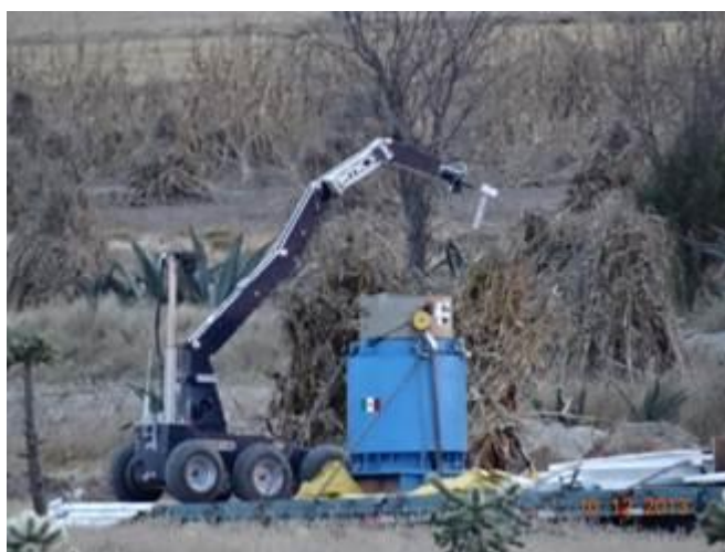
Fig. I-156. Placing the source in the container using the robot (Credit: CNSNS).
