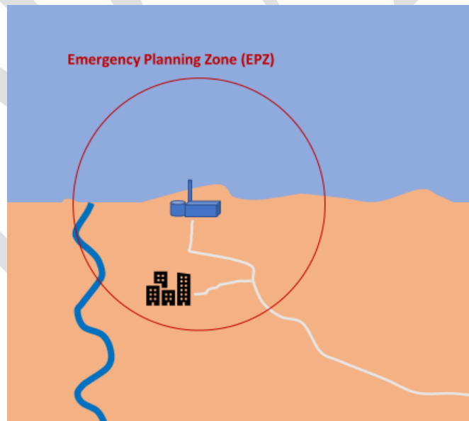
FIG. 2. Example of an unsuitable site — a physical barrier (river) preventing construction of an alternative evacuation route in another direction — site unsuitable if a bridge is not constructed or alternative evacuation route.
