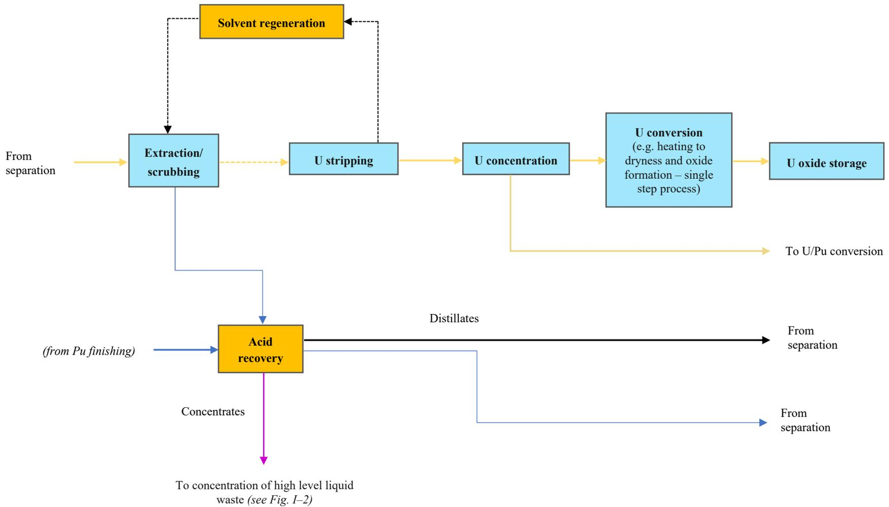
FIG. I-3. Uranium finishing at a reprocessing facility.
