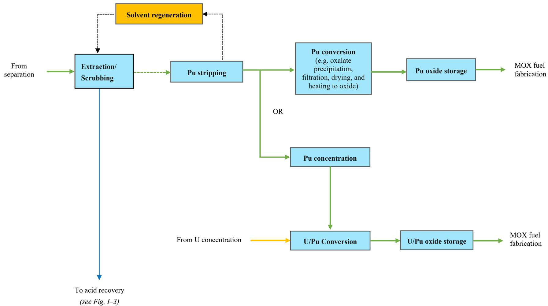
FIG. I-4. Plutonium finishing at a reprocessing facility.
