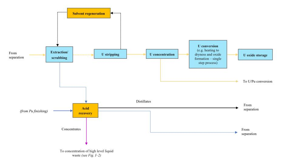
FIG. I–3. Uranium finishing at a reprocessing facility.
