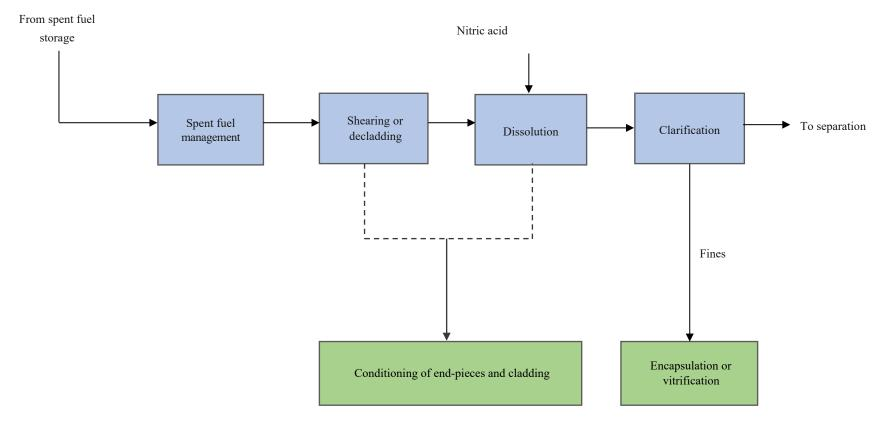
FIG. 1–1. Main process routes at the head end of a reprocessing facility.
