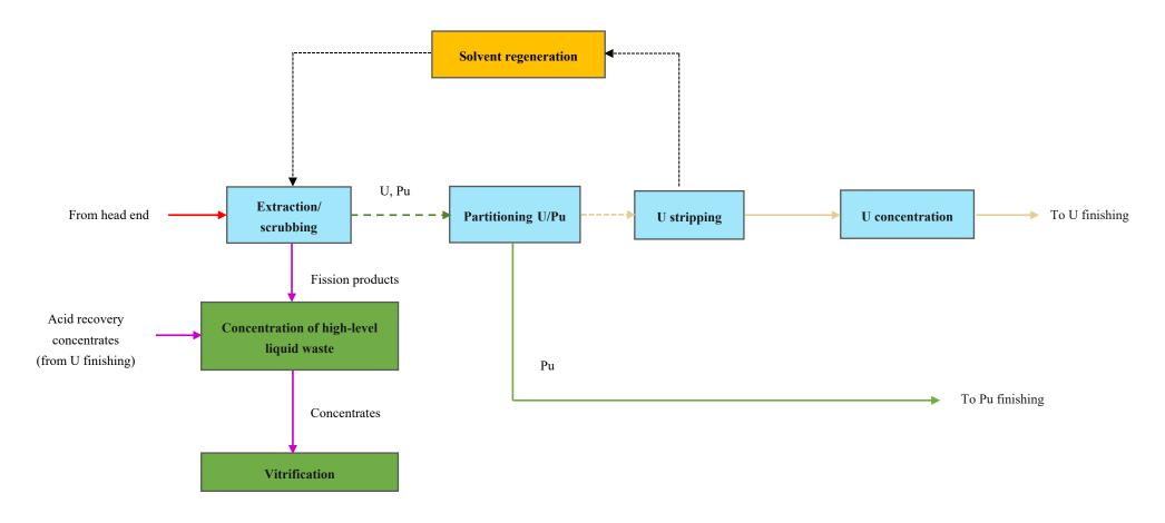
FIG. 1–2. Separation of uranium and plutonium at a reprocessing facility.
