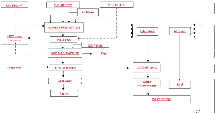
Fig. I–1. Typical process routes in a MOX fuel fabrication facility.
